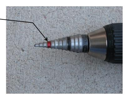
Using the bracket as a template, mark the mounting hole locations on the radiator core support and carefully drill four 3/8" diameter holes.
