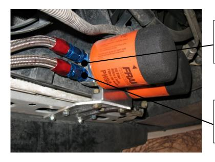
CENTER PORT – CLEAN OIL OUT TO THE BY-PASS ADAPTER (MARKED "OUT" ON THE CASTING)
