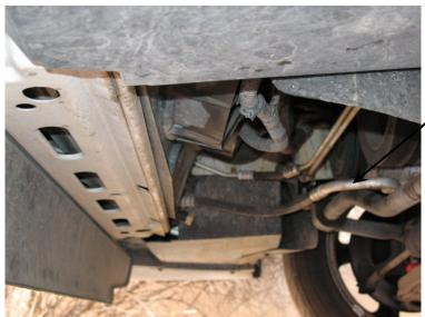
IT WAS NECESSARY TO BEND THIS AC LINE TO MAKE ROOM FOR THE OIL FILTERS – THE ALUMINUM TUBING BENDS EASILY - BE CAREFUL NOT TO KINK OR BREAK IT!
